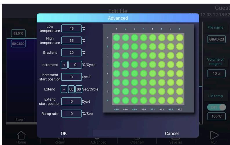
Figure 11. Set the Vertical Gradient
